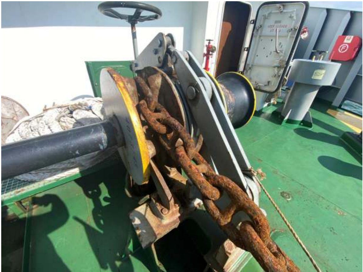
035. Port windlass winch.
