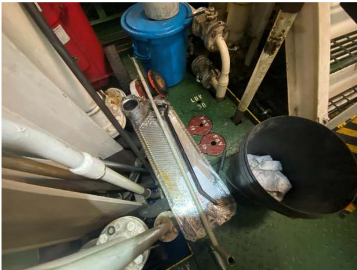
125. LO cooler plates dismantled from aux. engine no. 2.
