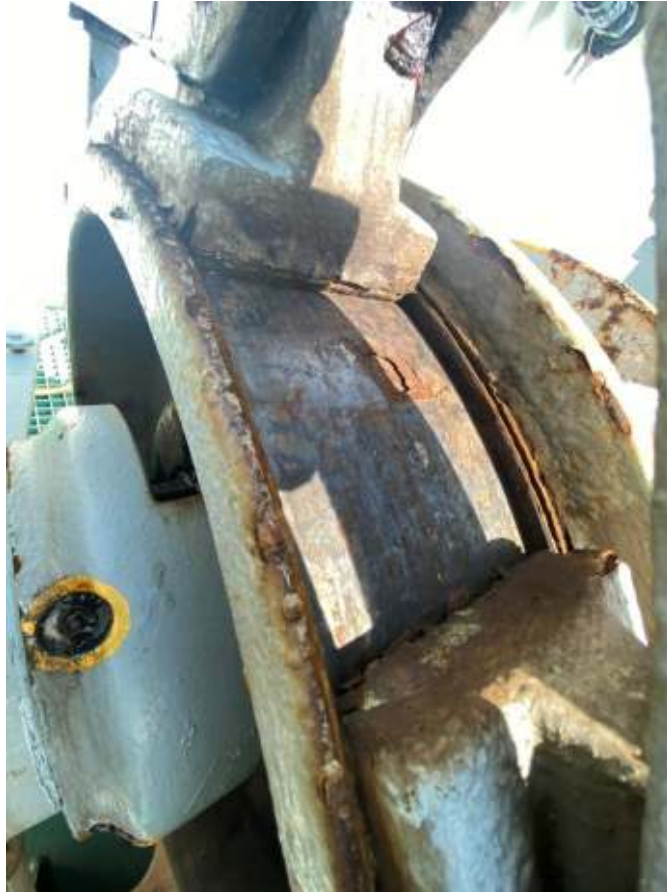
037. Windlass brake pad and drum.
