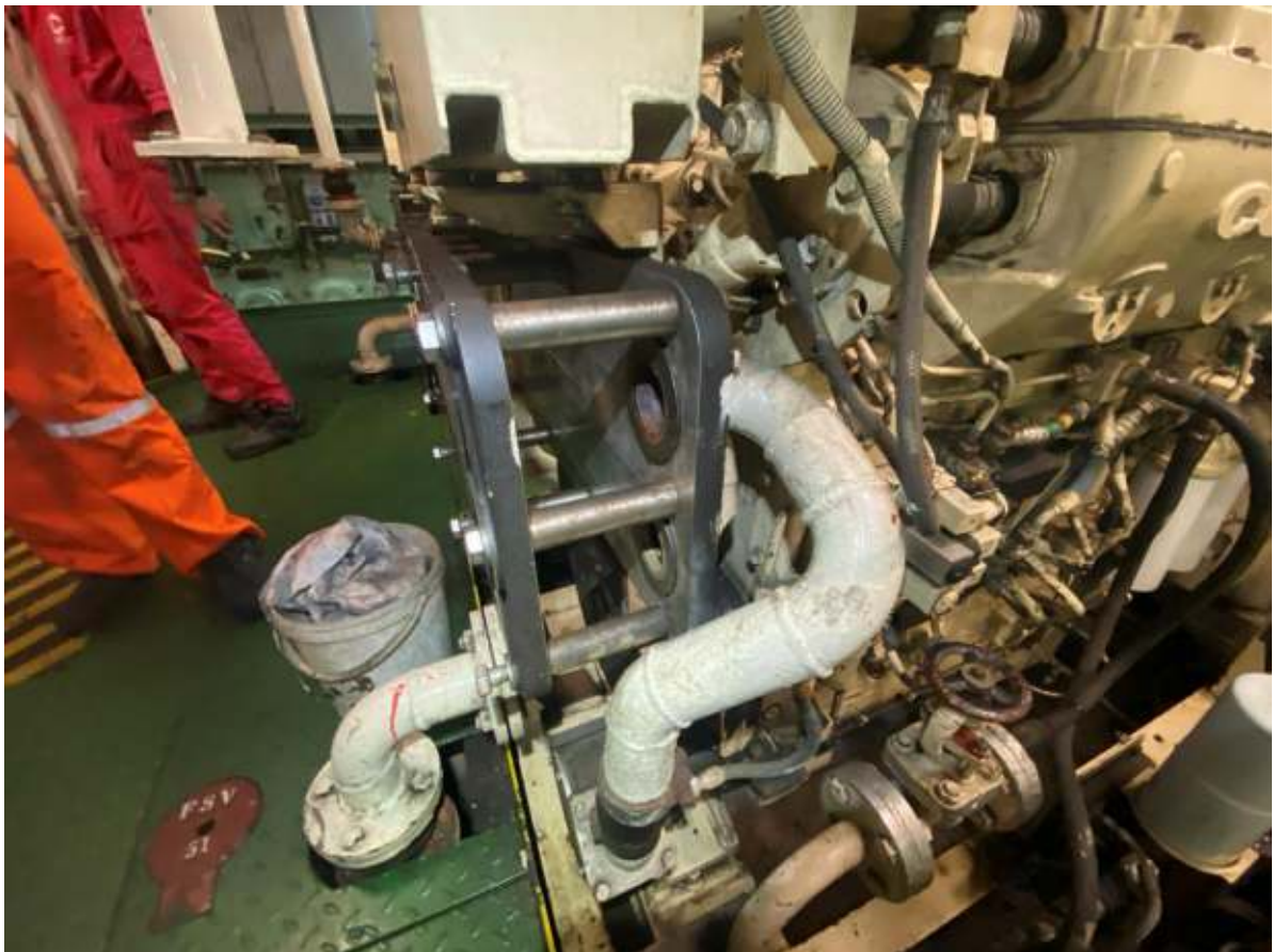
124. Aux. engine LO cooler removed.
