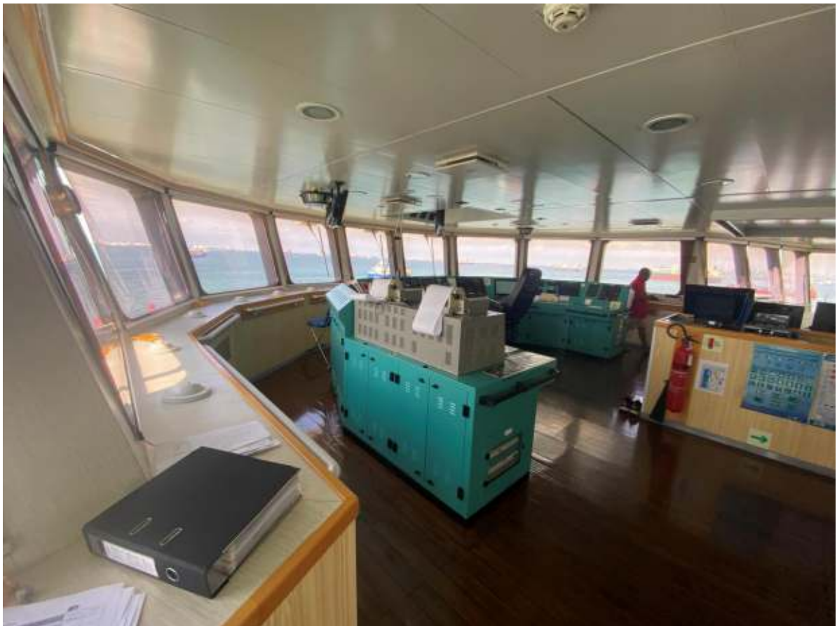
084. Wheelhouse navigation/ steering console.
